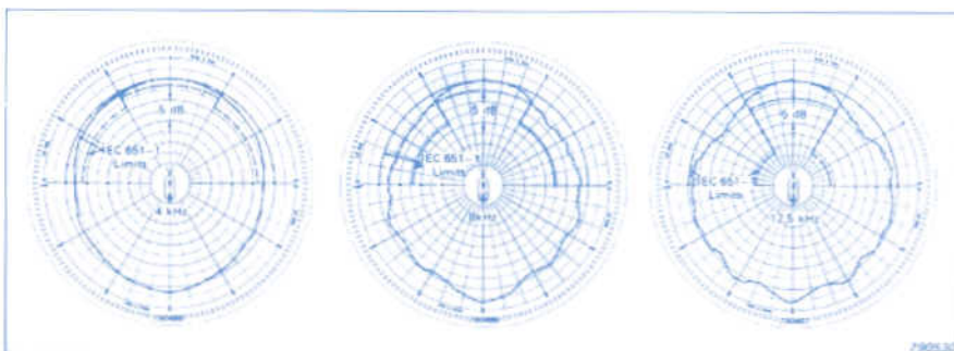
Fig. 5. Directional characteristics of the combination shown in Fig. 1 (Microphone Type 4149)
