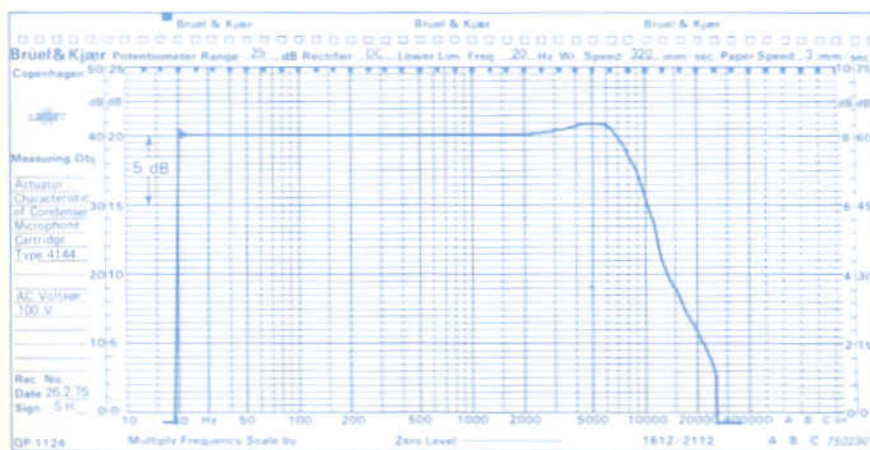
Fig. 12. Microphone frequency characteristic recorded by means of the set-up shown in Fig. 11
