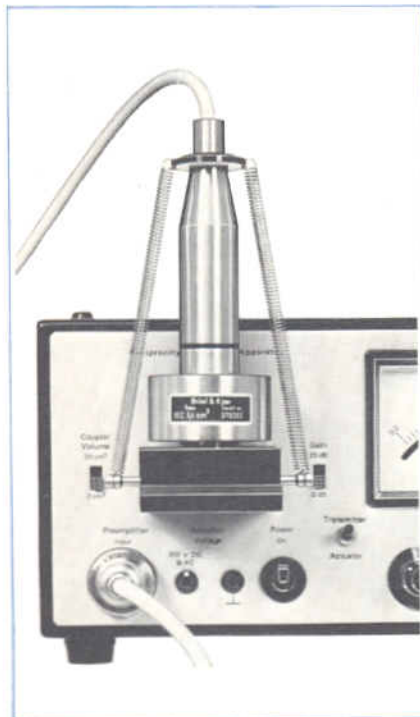
Fig. 5. Type 4143 fitted with 1" microphones, preamplifier and 3.4 cm 3 IEC plane wave coupler
