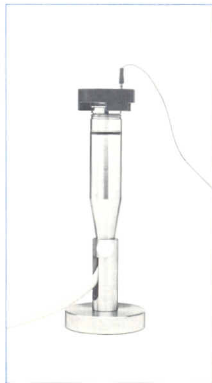
Fig. 13. 1" Condenser Microphone mounted with Electrostatic Actuator UA 0023 and preamplifier placed in Adaptor UA 0028 and on Stand DB 1689 for calibration
